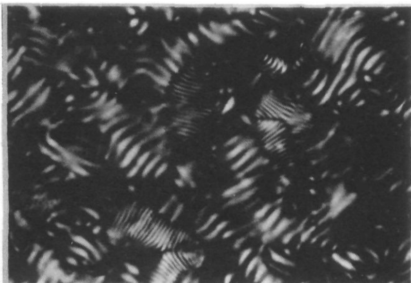
Figure 6. Texture of coexistent cholesterics. Domains with smaller fingerprint texture, Ch L , are separated by sharp boundaries from the large fingerprint pattern, Ch C , 0.3 mm thick, 60×, crossed polarizers.
