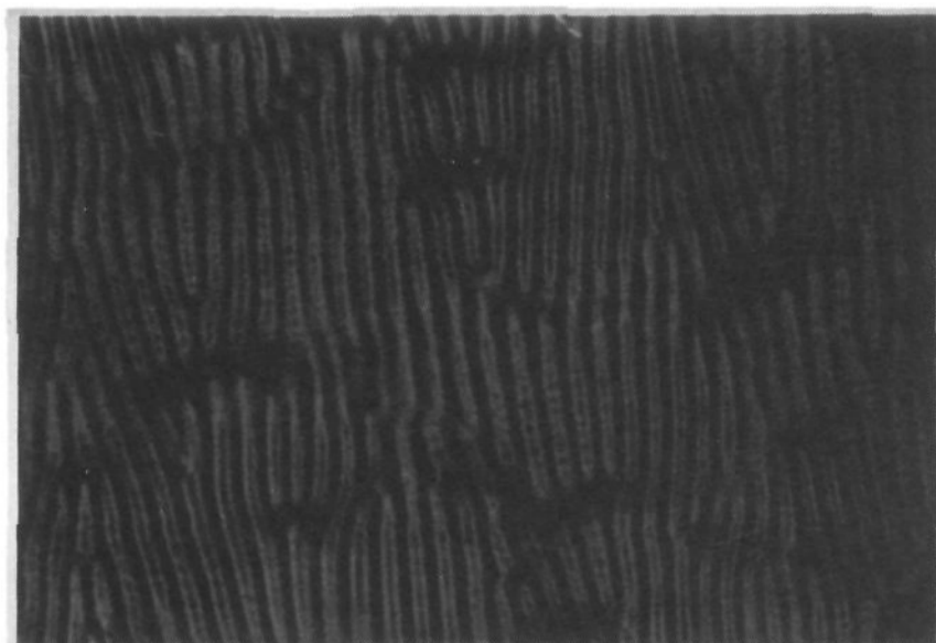
Figure 7. Texture obtained after spinning the sample of Figure 6 vertically to the magnetic field for 8 h. Spinning axis coincides with the long edge of the picture, 0.3 mm thick, 60×, crossed polarizers are slightly rotated.
